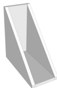
A cushioning corner for simultaneous padding and fixation of a painting in a crate.
