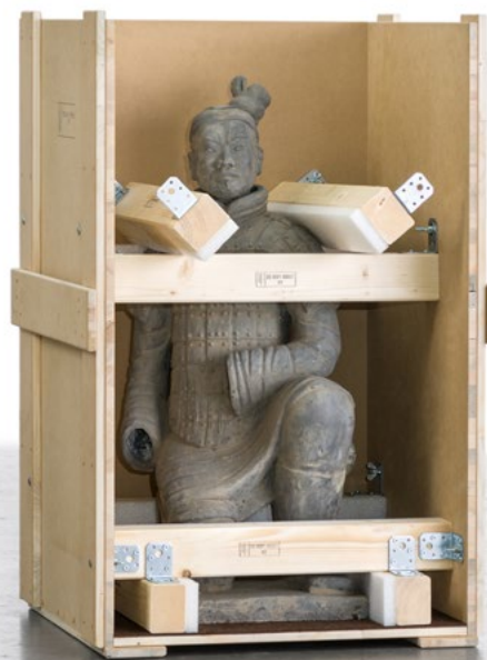
Bar fixing in a crate. Two beam annuli and padded contact areas secure the sculpture. The beams are connected via metal angels and wings screws with the crate (crate: object crate / "hasenkamp standard").
